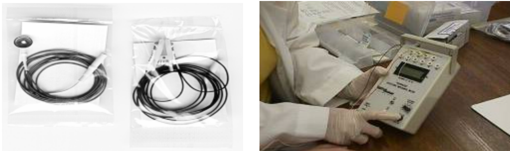
Figure 4. (Left) Recording electrode; reference electrode Figure 5. (Right) Impedance meter; (Grass Instruments model F-EZM5)
