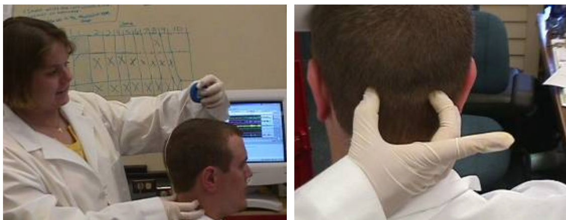
Figure 3. Learning in this investigative laboratory will include the following: Left picture: Measuring to place EEG electrodes at the O1 and O2 Occipital positions on participant's scalp. Right picture: Approximate location for O1 and O2 electrode placement
